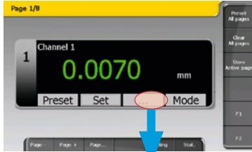
To do this, use the « ... » button (also accessible through the Setting → Measurement Setting menu).
