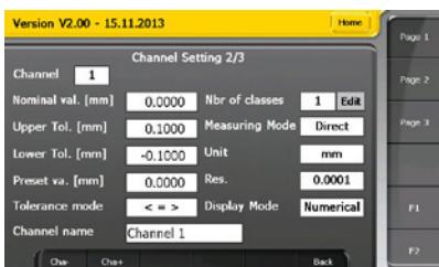
Configuration of a channel's measurement parameters, such as tolerances or preset values.
