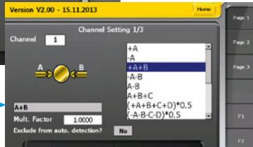
Allocate the instruments to be used to carry out the calculation. Select the instruments for channel A then channel B.
