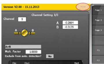
By moving the instrument, the value will also move on the A and B displays. This enables one to check the instrument selection. To finish press « Home » to exit the configuration menu.
