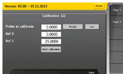
**Page 2:** allows a linearity correction using 2 to 25 points. The number of points and the measurement step can be entered. The value of the calibration blocks can be modified during the calibration procedure if it does not correspond to the measurement step.
