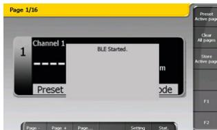
Connect the Bluetooth receiver to a USB port on the D300S then switch on the unit. The connection activates automatically and the following message appears when the unit starts up.
