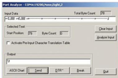
Type in the "output" window the retro-command " ? " followed by the "CR" carriage return ASCII (13) character to display the value of active channels.
